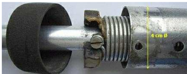
Damage due to a dirty (vintage) trap and exceeding the power.
