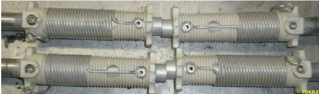
The rivets replaced by stainless steel bolt and nut.
