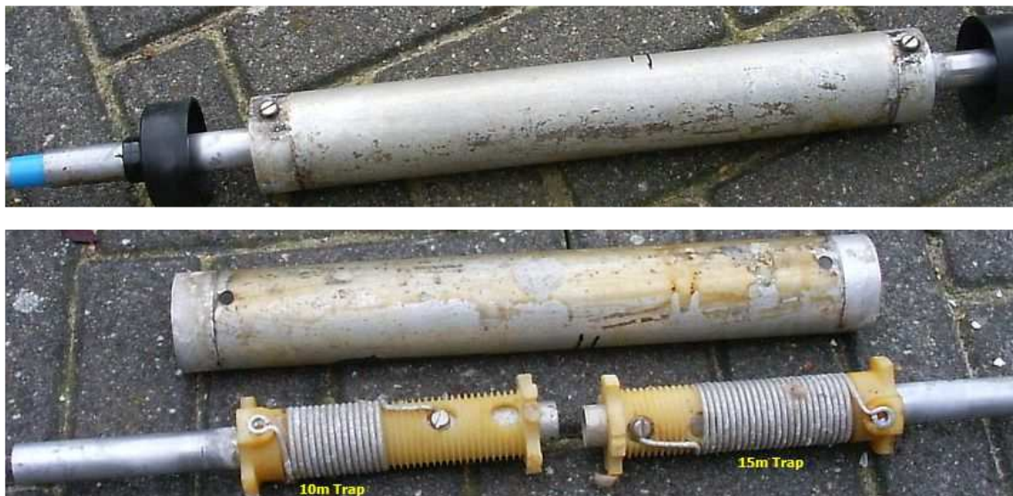
Fritzel 15 en 10 m traps from a 3 bands dipole of a FB13, FB23 of FB33 (< 1983).
